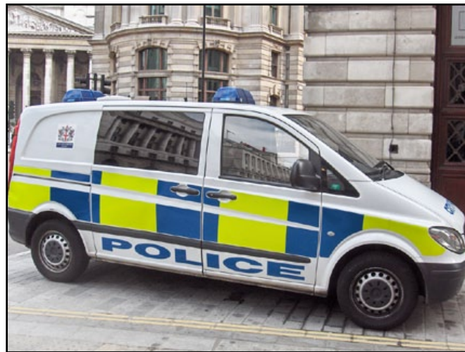
Figure 6—Retroreflective Half-Battenburg pattern.
