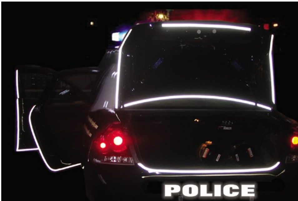
Figure 14–Edge markings on a patrol car.
